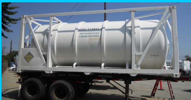
(2) 20 ft ISO LOX Tanks
